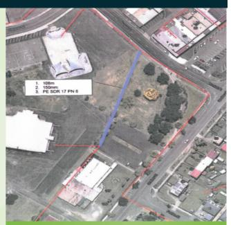
Failures in the AC (asbestos cement) sewer pipes near geothermal areas has prompted emergency repairs and an evaluation of the entire line
