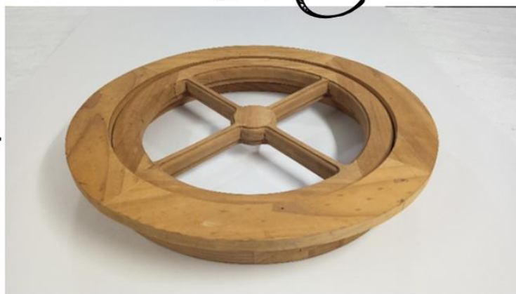
Wooden pattern of a ring gear made at Tasman mill circa 1966. Kawerau Museum 2022.185
